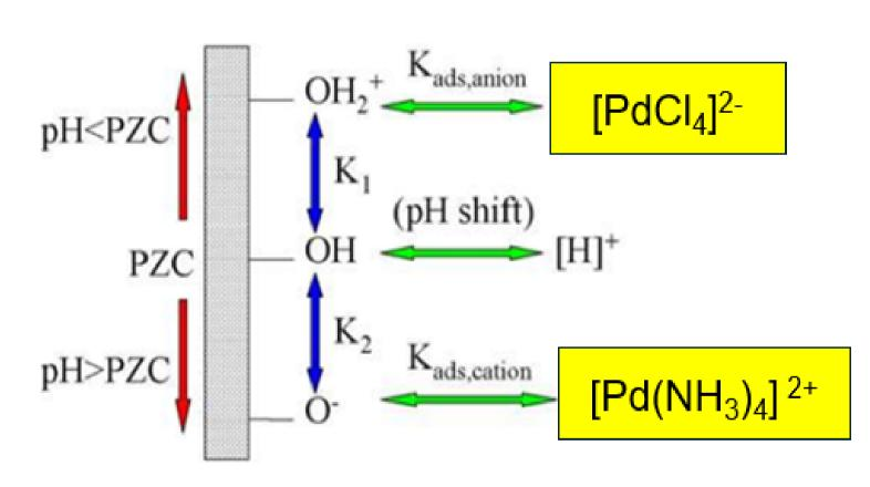
Unless otherwise stated, cationic chloride-free palladium precursor (palladium tetraamine nitrate) was used for all synthesis, at pH 10.5-12
